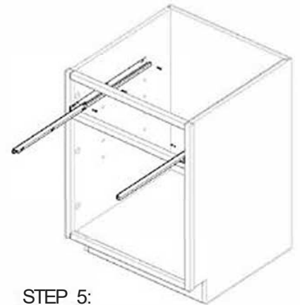
STEP 5: Slide the Drawer Slide from the Faceframe until the drawer slide is aligned with the faceframe, then fasten into pre-drilled holes.
